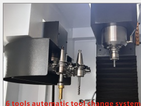
6 tools automatic tool change system
