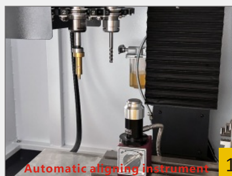
6 tools automatic tool change system
